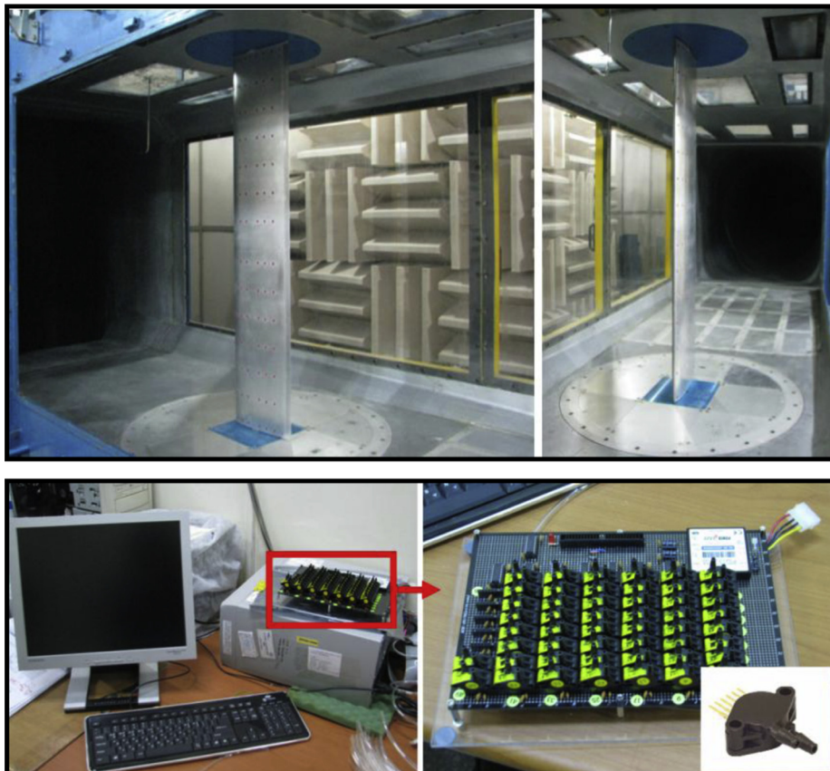
Fig. 6. The KIER aerodynamic tests in the Chungnam National University anechoic wind tunnel (upper; test section, lower; pressure tap sensors).
